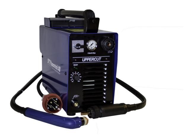
**UPPERCUT** is a 120A portable air-plasma system with extremely high performance in relation to its low weight, the power source weighs only 18 kg and can cut up to 45mm thickness. With air plasma systems you can cut mild steel, stainless steel, aluminum, brass, copper and other electrically conductive materials.
