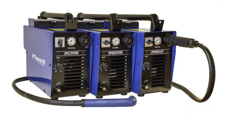
**SPLITFIRE, SPEEDFIRE** and **UPPERCUT** are portable air-plasmasystems with extremely high performance in relation to their low weight, the power sources with 80, 100 and 120A only weighs 17-18 kg and cut up to 25, 35 and 45mm thickness.
