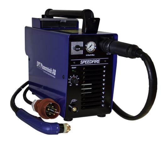
**SPEEDFIRE** is a 100A portable air-plasma system with extremely high performance in relation to its low weight, the power source weighs only 17 kg and can cut up to 35mm thickness. With air plasma systems you can cut mild steel, stainless steel, aluminum, brass, copper and other electrically conductive material.
