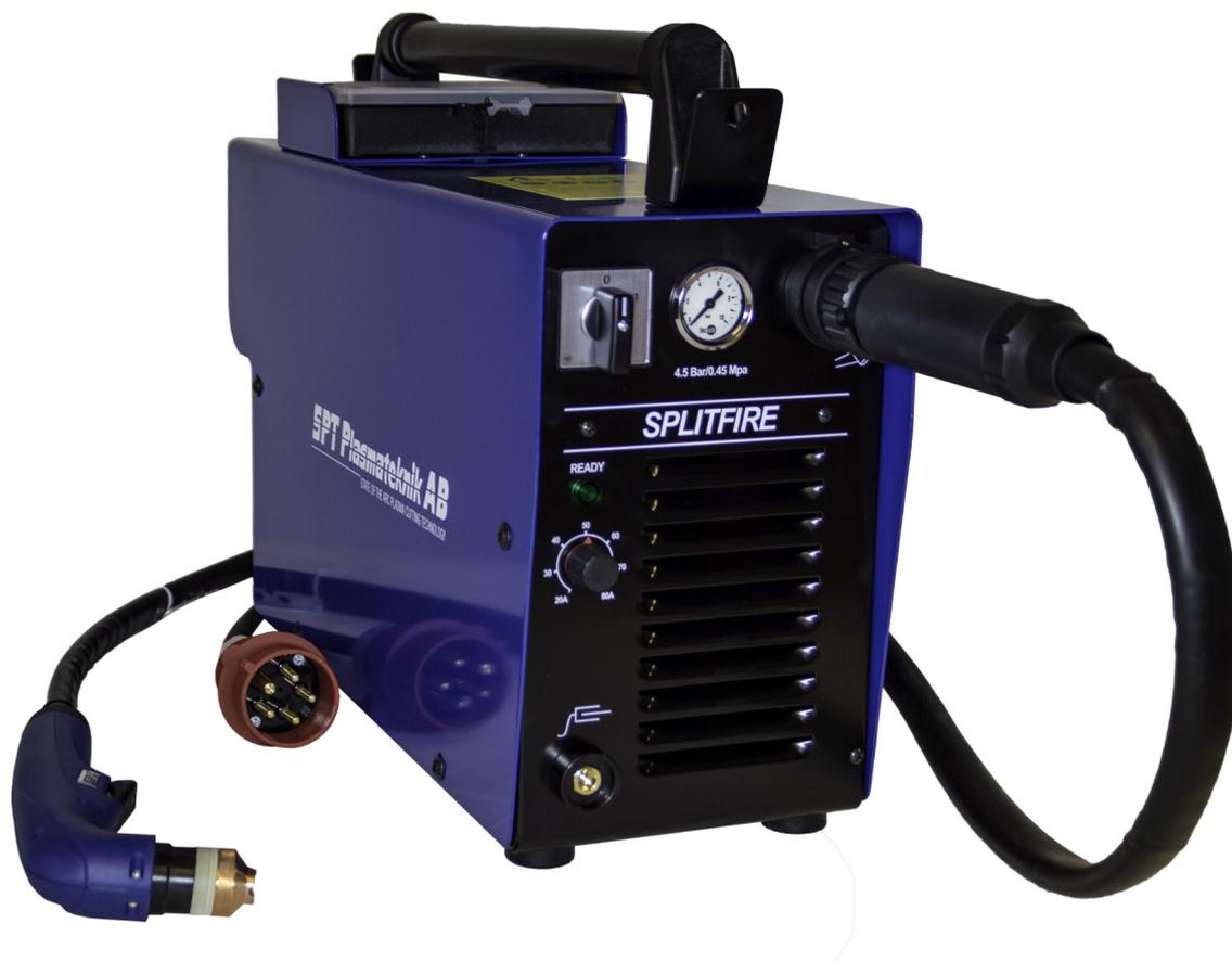
**SPLITFIRE** is a 80A portable air-plasma system with extremely high performance in relation to its low weight, the power source weighs only 17 kg and can cut up to 25mm thickness. With air plasma systems you can cut mild steel, stainless steel, aluminum, brass, copper and other electrically conductive materials.
